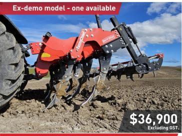
FARMCHIEF SSDR HEAVY DUTY DEEP RIPPER 3m wide, 7 legs, 850mm clearance, dual spiked hydraulic roller
